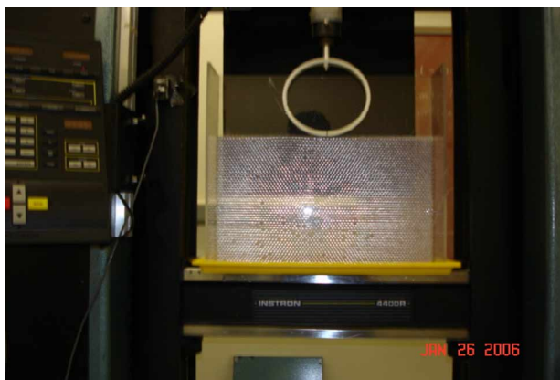
Figure 2. Indentation experiment setup, with the cylindrical indenter at the top, on an Instron machine. The indentation is done at a chosen rate of 0.1 in. per minute by pushing down the cylindrical indenter.
